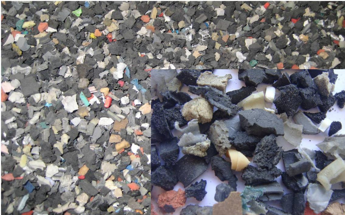
◀ 3 Elastomer fraction after separation by a hamos RSS line
