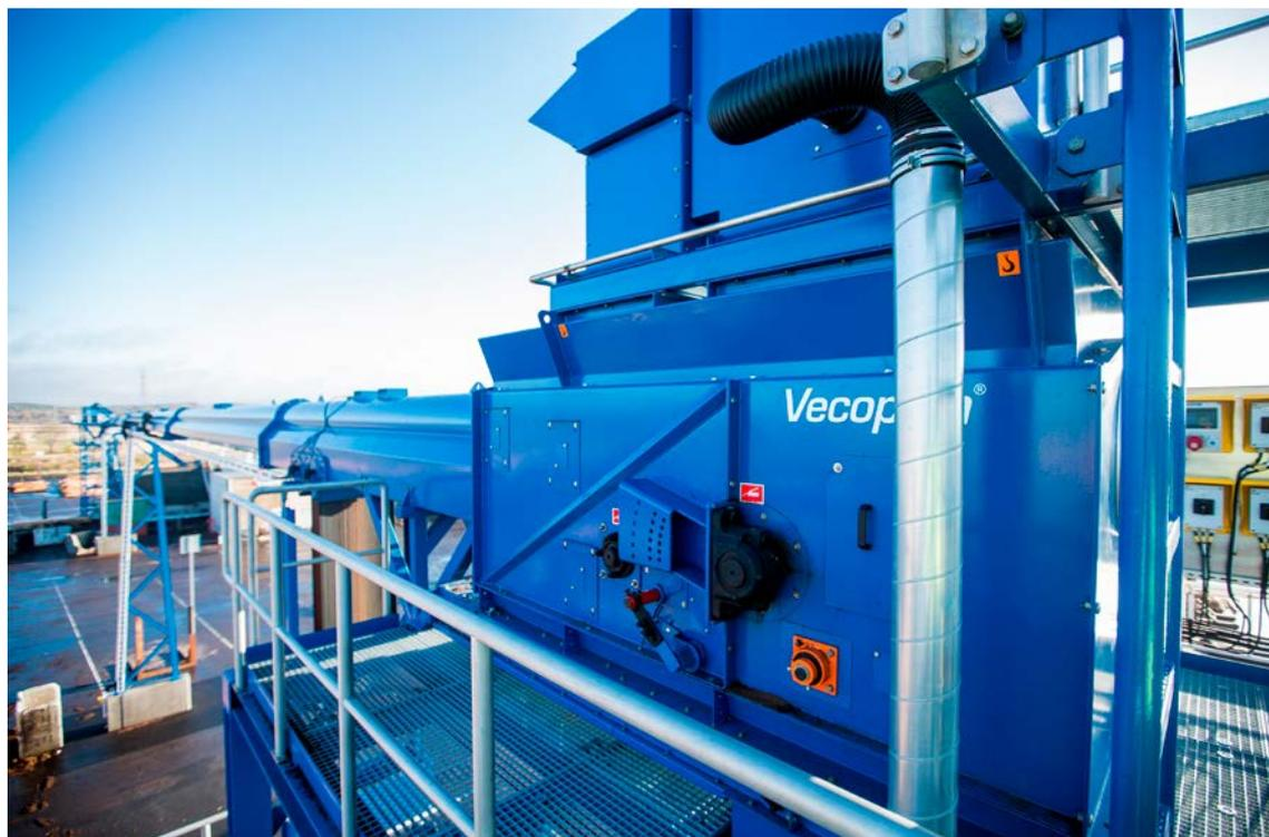
The pipe belt conveyors of the VecoBelt series transport bulk material without losses
