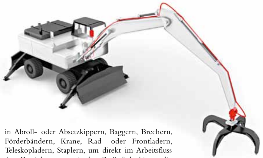
▲ Excavator scale with the weighing electronics in the driver cabin and the measuring element at the grapple
