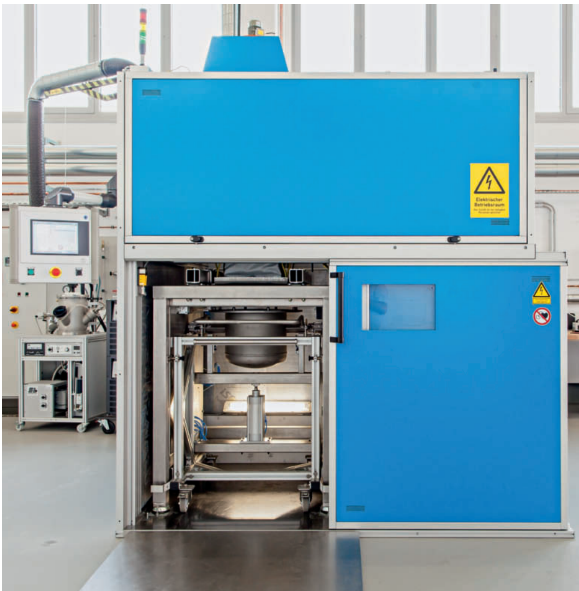
◀ 2 EHF 400 shock wave fragmentation system of the Fraunhofer IWKS Project Group in Alzenau
